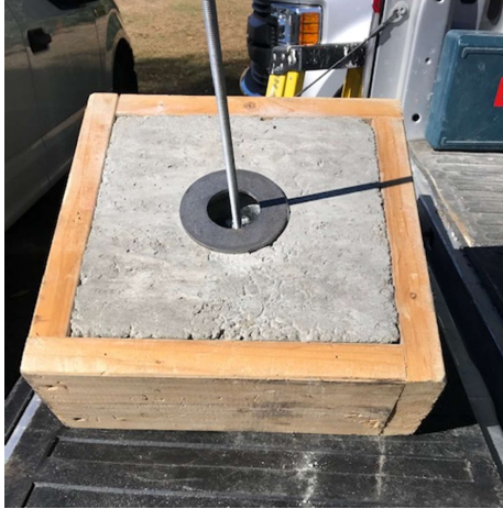
Setting up for the test, rod is installed and ready for the hydraulic ram
