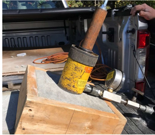
The hydraulic ram is in place and ready to begin test
